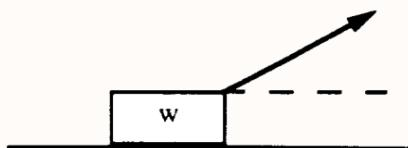
A block of weight  $W$  is pulled along a horizontal surface at a constant speed by a force  $F$ , which acts at an angle  $\theta$  with the horizontal, as shown above. The normal force exerted on the block by the surface has magnitude of
